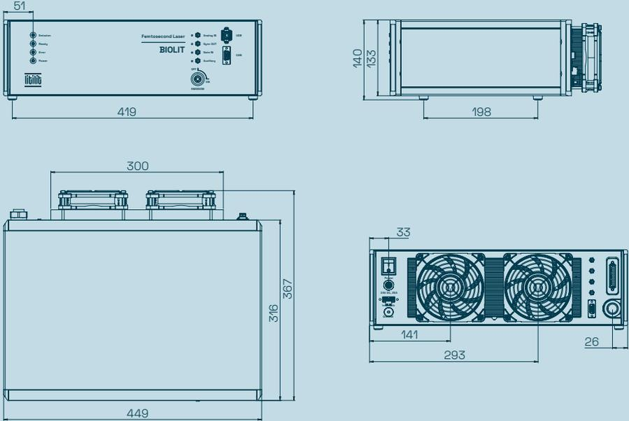
Drawing of Biolit 2 control unit (in mm)
