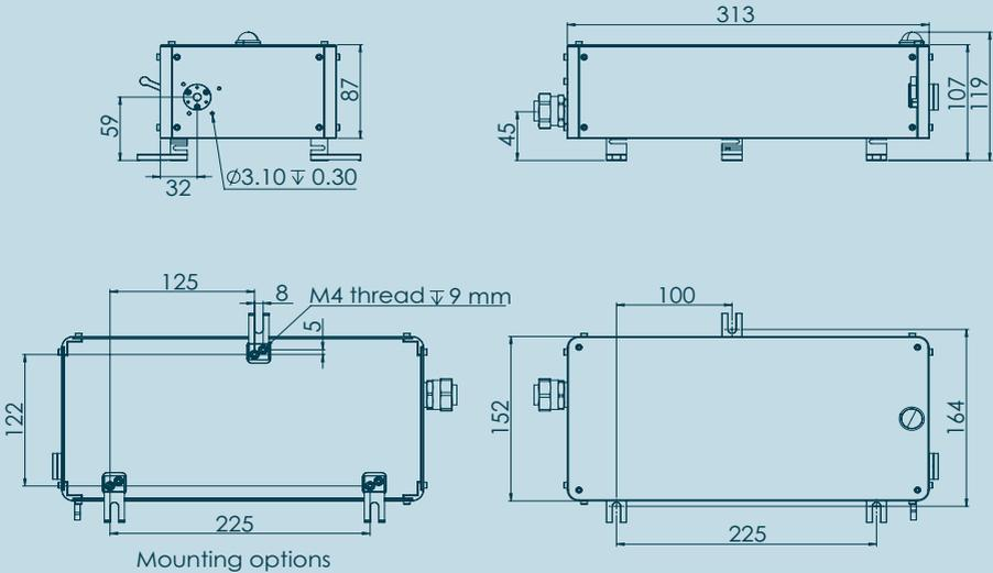
Drawing of Biolit 2 laser head (in mm)
