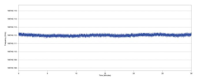
Model 872A-NIR wavelength measurement results for a 1532 nm acetylene-locked laser over a 30-minute time period. Standard Deviation is 191 kHz.
