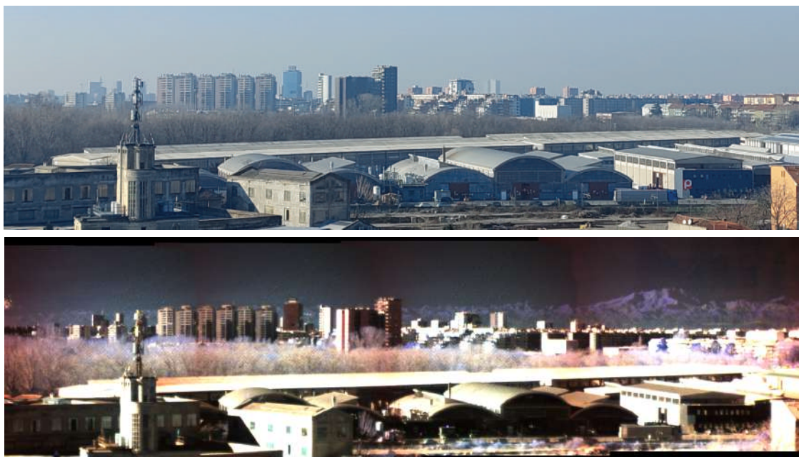
Photo taken with a camera False RGB image (R=1925, G=1405, B=1280 nm) obtained from a hyperspectral image acquired with HERA eSWIR
