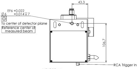
Working distance between input aperture plane to measuring plane is about 41 mm.
