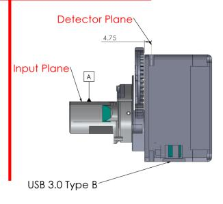
Optical distance from Input plane A to Detector Plane: 49 +/- 0.5
