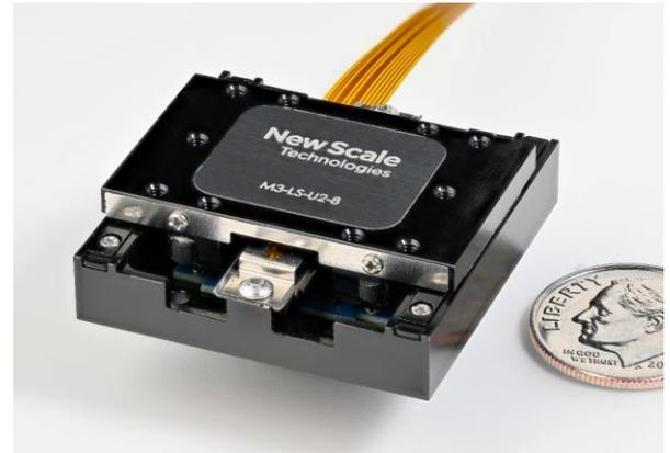
**The M3-LS-U2-8 Linear Smart Stage** is an ultra-compact positioning stage with sub-micrometer resolution and absolute encoding. *All electronics are built into the stage* for simple system integration. This model features power-off hold, high speed, and is cost-effective for high volume manufacturing.
