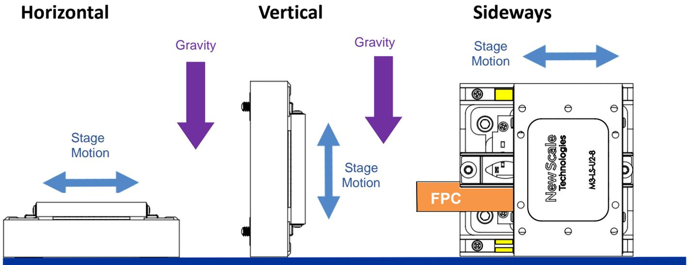
Note: Sideways Orientation Requires Flat Bearing Race Located at Top of Stage (As Pictured Above)
