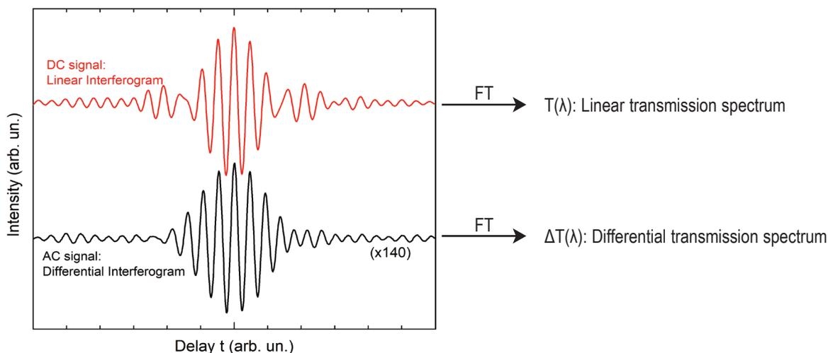
**FIGURE 2:** Examples of the linear and differential interferograms, which are measured simultaneously.
