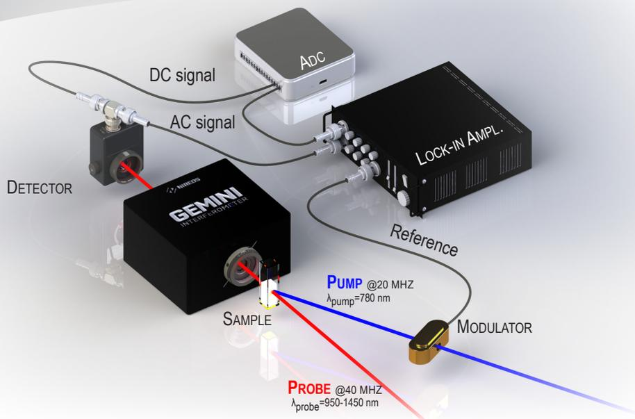
**FIGURE 1:** Experimental Setup for Pump-Probe Spectroscopy using the GEMINI Interferometer.
