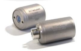
EOT's TORNOS Compact optical isolators are designed for wideranging end applications where optical feedback can adversely affect laser performance. TORNOS Compact isolators provide high transmission in the forward direction while strongly attenuating light traveling in the reverse direction, protecting lasers from the deleterious effects of back reflections.
