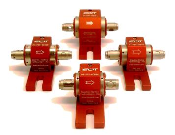
EOT's TORNOS Faraday Rotators rotate the plane of polarized light 45° in the forward direction and an additional 45° of non-reciprocal rotation in the reverse direction while maintaining the light's linear polarization. When placed between crossed polarizers, a Faraday rotator becomes an optical isolator.
