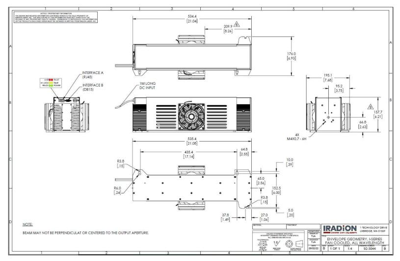
\*Note the drawing above is of an Infinity Fan cooled laser.
